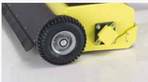
Soft rubber wheels that do not damage the grass, anti-puncture. They have ball bearings and are mounted on an axis of 20 mm in diameter.
