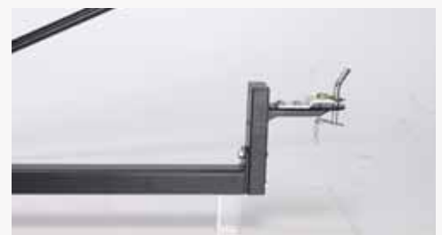
Adjustable helm attachment to facilitate coupling with any type of tractor or quad.
