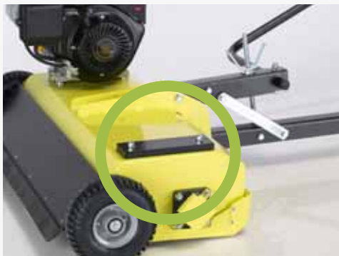
Balance ballast: to balance the weight of the motor placed on one side of the machine, on the opposite side there is a ballast (different depending on the type of motor chosen).
