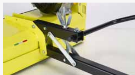
Working height adjustment system. From sitting on the tractor / quad, the lever can be lifted by the lever so that the knives do not touch the ground.
