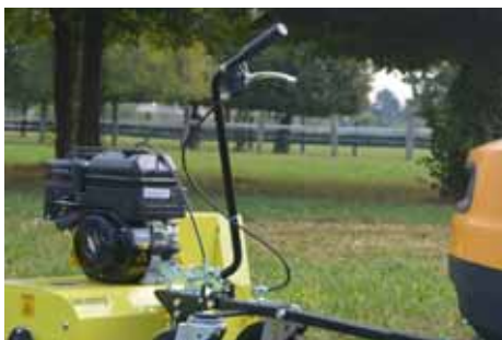
Lifting handel and automatic starting of cutting system.
